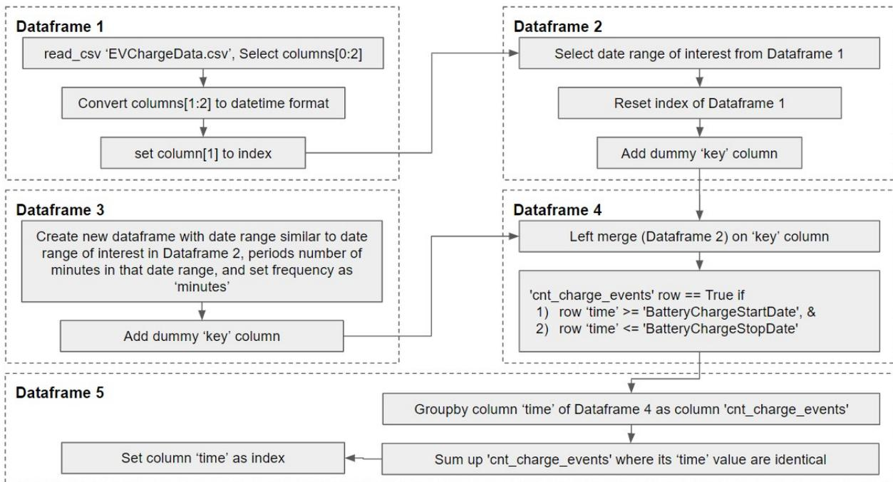
Figure 1 Flowchart of proposed procedure for start-stop data transformation process.
