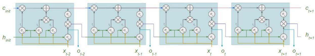
Figure 6: Visualization of four units of LSTM cells in sequential single layer configuration
