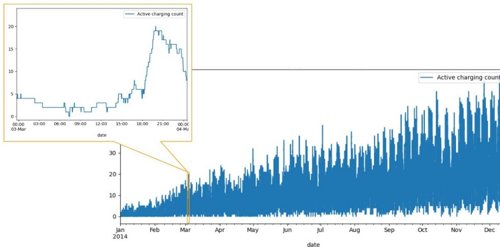
Figure 4: Feature engineered continuous time series data generated from the start and stop charge data sourced from the My Electric Avenue Project
